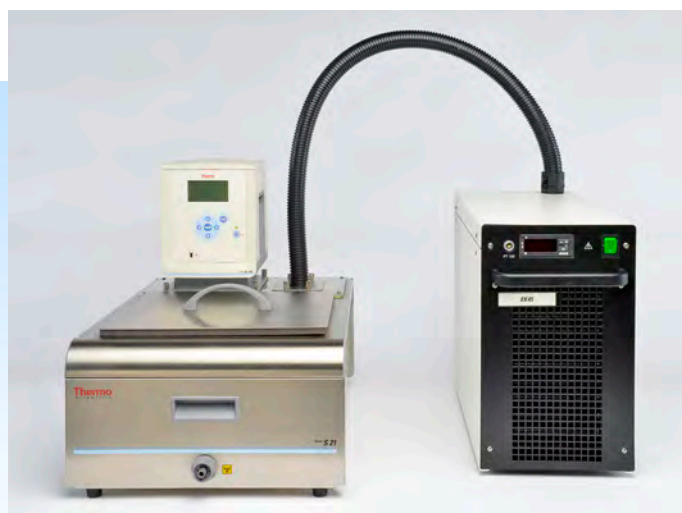
Thermo Scientific™ EK45 Immersion Cooler with a SAHARA S21 Stainless-Steel Heated Bath Circulator
