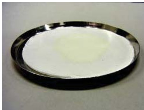
After the extraction of moisture, a thin yellow grease stain remains
